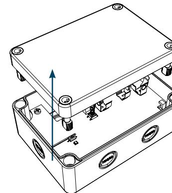
Remove the lid from the back box, removing the screws on the corners.
