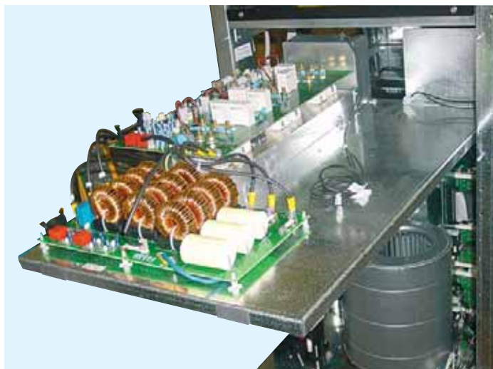
Sentry Multistandard with Active Filter (internal view)
